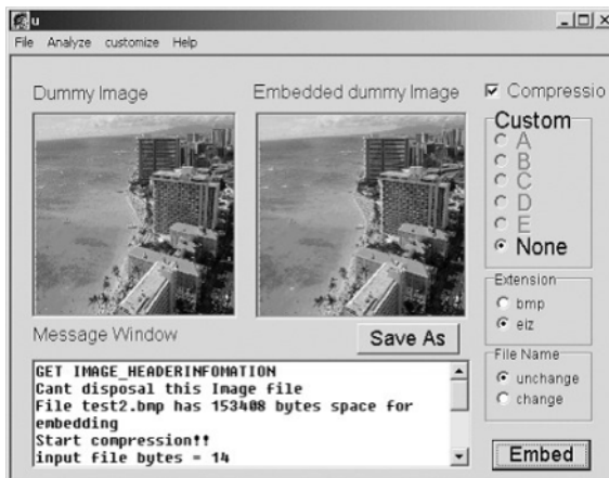
Figure 6.13 Digital Picture Envelope screen showing both the original image and the image that has data hidden in it.
