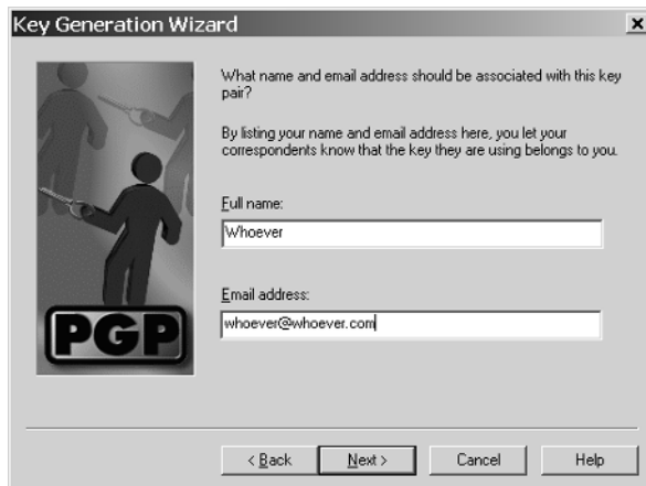
Figure 2.3 The first step in the process of generating a key is associating it with an email address.
